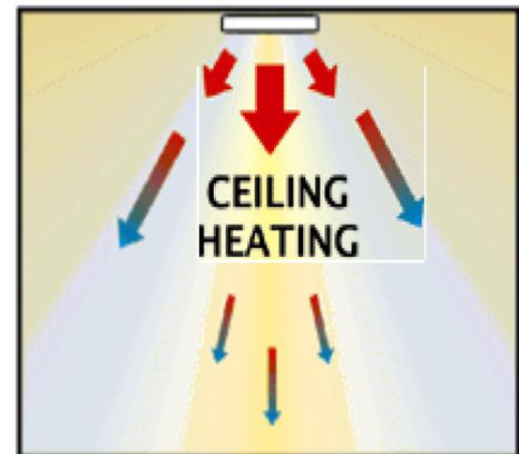
Ceiling mounted heaters warm the upper body only, leaving feet cold.
