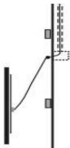
3. Hang mirror as per holes & domes instruction supplied with the mirror. Feed the excess wire into the wall cavity during installation.
