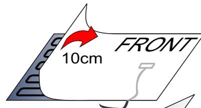
3. Flip the demister pad again, adjust it to the marked position, use a dry cloth and press the bonding foil on to the back of the mirror.
