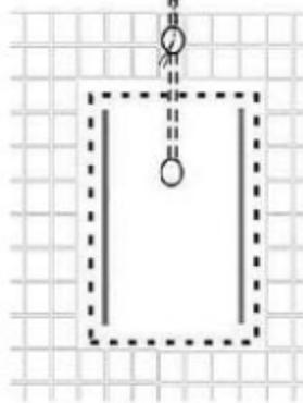
4. Thread a wire through an electrical conduit or pipe. Connect the power cord of the demister to the wire. Fix the mirror onto the wall while pulling the wire through at the same time.
