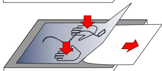
5. Mark and transfer dimensions of the mirror and location of the power cord.
