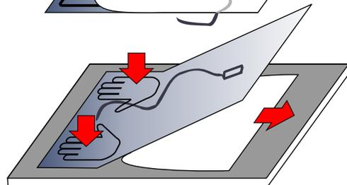
4. Slowly peel the protection film back, while pressing and rubbing the bonding foil onto the back of the mirror with the dry cloth. It is easiest to use two people, one peeling and one pressing.
